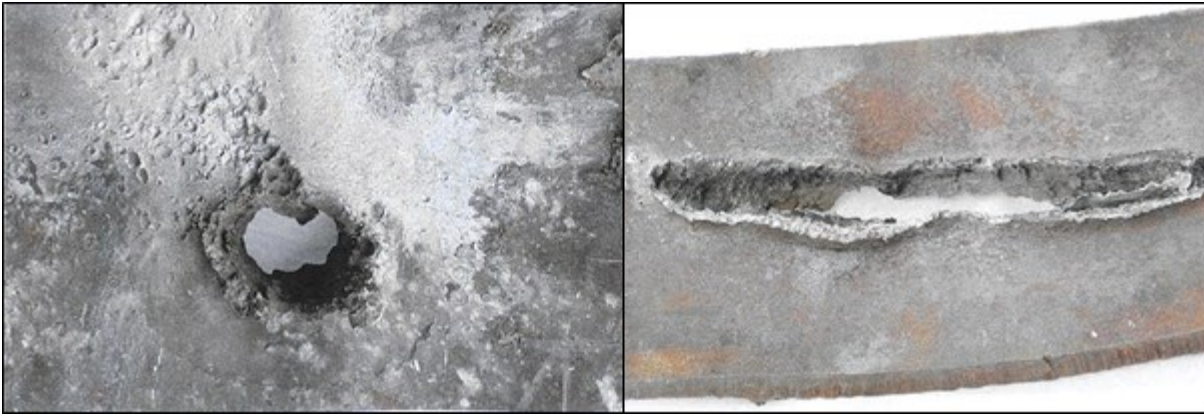
Figure 1: Holes punched through 1 inch steel plates from the explosive energy of shaped charges: Cone shaped charge (left); Linear shaped charge (right).
